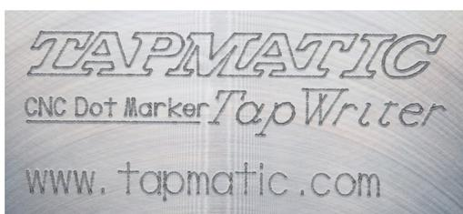
Marking plane 3mm, 850 RPM,
