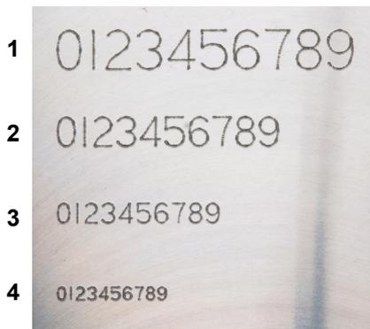
1. Character height 6mm, marking plane 2.5mm, 850 RPM, feed rate 500 mm/min.
