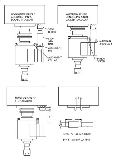
Step 2. Adjusting Alignment collar: With tapping attachment in machine spindle and with spindle oriented for an automatic tool change, bring the slot in the collar in to position where it is directly over the alignment pin. There is a key packaged with the wrenches to help line this up. Then tighten the collar securely. After checking clearance with tool changer and in tool magazine area make several automatic tool changes.
