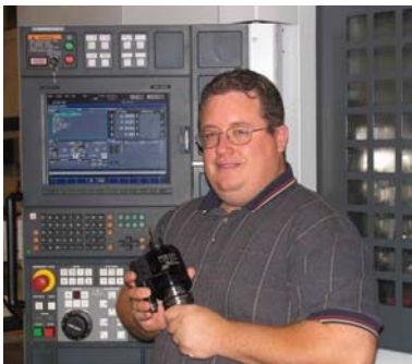
Eric Barnard holds the Tapmatic self-reversing tapping head that drastically reduces cycle time for finishing holes on the aluminum parts produced in high volume on the HMC behind him.
