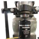
Always mount a torque bar to hold the tapping attachments stop arm from rotating. The torque bar must be mounted securely to the table or quill of your machine. The torque bar installation must be stronger than the largest tap in the capacity range of your tapping attachment. The surface of the torque bar must be smooth to allow the stop arm to slide freely when feeding in and out of the hole. Order Tapmatic Torque Bars shown.
