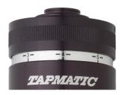
Setting the pre-selective torque control: The torque control helps prevent tap breakage, especially when tapping blind holes. Tightening the cap down to the higher number settings on the reference scale increases torque. To set the torque, use a new tap and begin with a low number (low torque) setting. Try to tap the hole.
