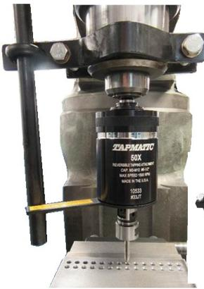
**Always mount a torque bar to hold the tapping attachments stop arm from rotating.** The torque bar **must** be mounted securely to the table or quill of your machine. The torque bar installation **must be stronger** than the largest tap in the capacity range of your tapping attachment. The surface of the torque bar **must be smooth** to allow the stop arm to slide freely when feeding in and out of the hole. Order Tapmatic Torque Bars shown.
