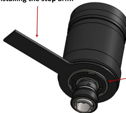
In order for the Tapping Head to reverse, the stop arm must be prevented from rotating.
