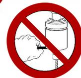
**5. Do not exceed the maximum speed for the tapping head:** Speed is a critical factor in tapping. Please always refer to recommended tapping speed chart.
