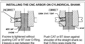
it leaves a gap between the shoulder of the straight shank and the bottom of the CAT or BT. When tapping a hole, the O-Ring compresses and the screw could become loose.
