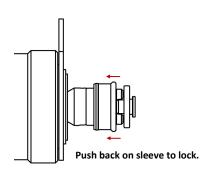
**Installing an ER collet into the ER collet adapter:** Always install the collet into the nut first. Make sure lip inside the
